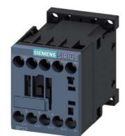
contactor AC-1, 18 A, 400 V / 40  $^\circ\text{C},$  4-pole, 230 V AC, 50/60 Hz, screw terminal, size: S00
