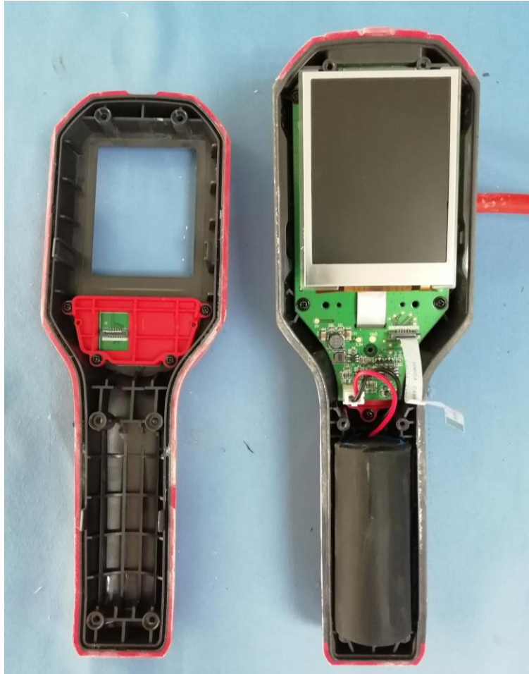
Photo 5 - Internal view after IP6X test
