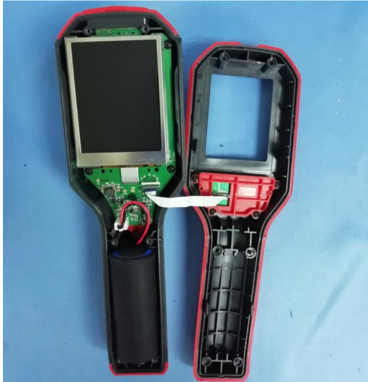
Photo 3 - Internal view after IPX5 test
